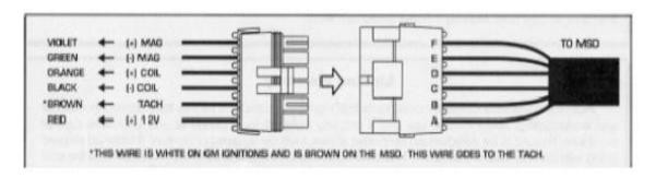
Above shows wiring order for connector installation on MSD 6AL and 6T Ignition Box
