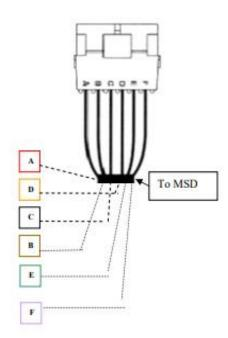
Rule 11.7 Wiring Harness 50-2053 for Ignition Wiring or Power plug diagram
